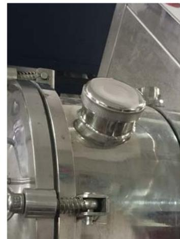
**Small cover on dye vat** is convenient to open for adding water, midway adding chemicals and taking samples.
